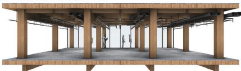
CLT / Concrete Composite System Full CLT structure acts as formwork for concrete screed and beams
